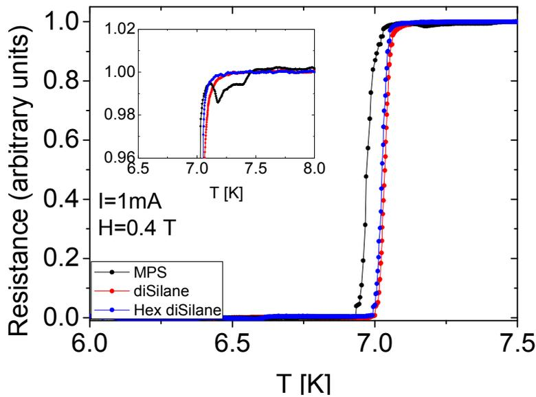
Figure 15: The resistance as a function of temperature for the three systems at 0.4T magnetic field applied: MPS (black), diSilane (red) and Hex diSilane (blue). The inset zooms in the peak effect area shows the peak effect for the MPS only.
