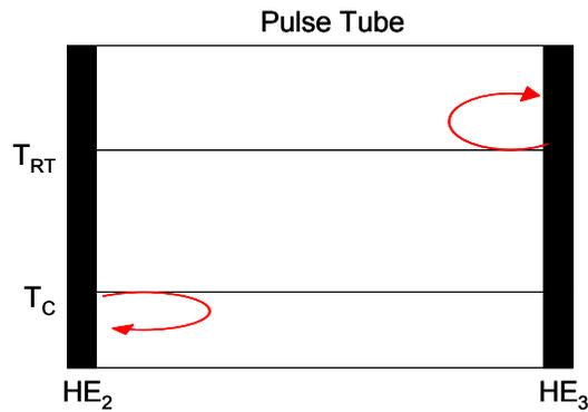
Figure 7: Gas elements enter in  $HE_2$  with temperature  $T_c$  and leaves with lower temperature. In  $HE_3$  the gas elements enter in room temperature and leave with higher temperature.
