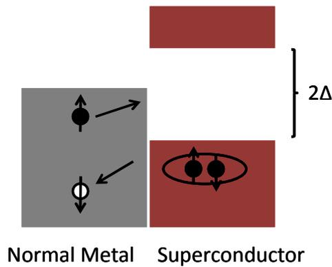
Figure 2: Schematic drawing of energy bands of the S/N junction. The Andreev reflection occurs at the interface by the propagating electron (black) and retro-reflection of a hole(white).
