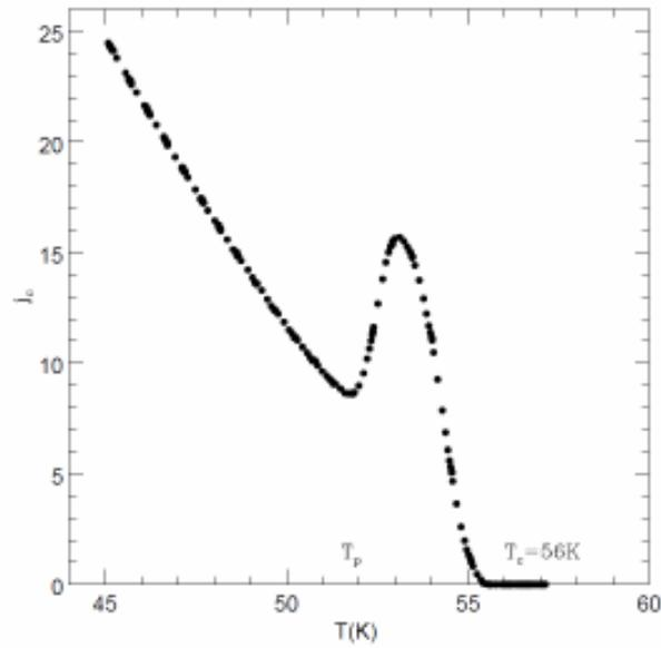
Figure 3: Critical current density of type II superconductor YBCO as a function of temperature. The peak in the current ascribed to the trapping of the vortices by the pinning landscape. This figure extracted from<sup>14</sup>.
