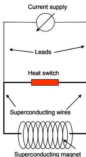
Figure 8: Drawing of the superconducting magnet system. The heat switch controls the persistence mode of the magnet.
