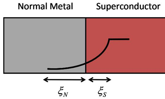
Figure 1: The diffusion of cooper pairs from the superconductor, on a scale of the coherence length, to the normal metal cause superconducting properties to the metal on the account of weakens the superconductor.
