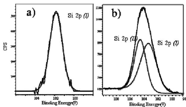
Figure 13. High resolution XPS spectra of Si 2p levels for a) OTS and b) diSilane samples.
