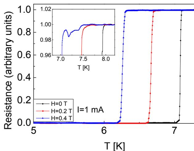
Figure 14: The resistance as a function of temperature for the bare Nb before the adsorption process in zero magnetic field (black), 0.2T magnetic field (red) and 0.4T (Blue). The inset shows the same data for the MPS molecule. A deep in the resistance or a peak in the critical current can be seen in 0.4T (blue).
