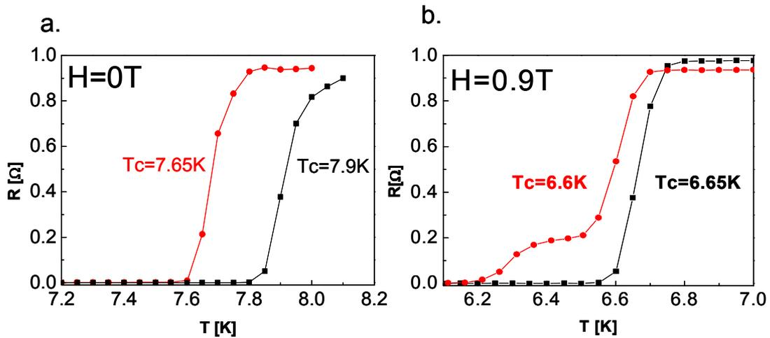
Figure 21: the resistance as a function of temperature for bare Nb (Red curve) and Nb after adsorption in diSilane molecules and 10 nm Au NP's deposition (Black curve) in the presence of perpendicular to the surface magnetic field in:  $H=0$  Tesla (a.) and  $H=0.9$  Tesla (c.). The measurements were performed in 2mA.
