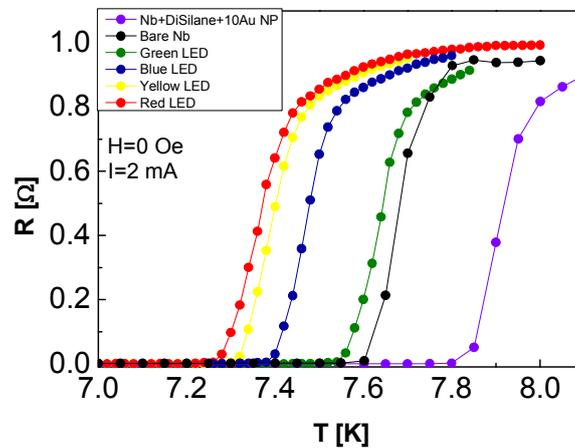
Figure 24: critical temperature results for: Nb adsorbed with diSilane molecules and 10 nm Au NP's (purple), Bare Nb film (black). The other results are LED emission in four different wavelengths: 526 nm (green), 470 nm (blue), 596 nm (yellow) and 660 nm (red).
