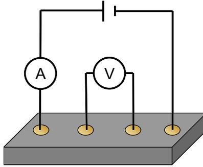
Figure 9: Four probe configuration scheme. Two of the wires are connected to DC current supply and two additional wires are connected to Voltmeter.
