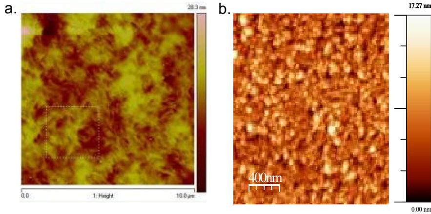
Figure 10: AFM measurement of the Nb surface fabricate by evaporation and sputtered techniques. The roughness of the evaporated sample is 3.5 nm (a.) and for the sputtered sample 3 nm (b.).
