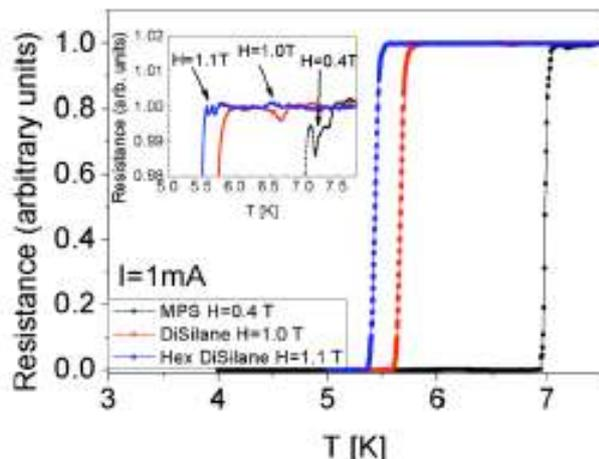
FIG. 4. (Color online) Normalized resistance of the Nb films as function of temperature for the three molecules used. The higher the magnetic field at which the peak effect is first observed the weaker the coupling of the molecule.
