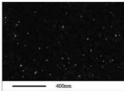
FIG. 2. HRSEM of the Nb surface coated with organic monolayer and 10 nm Au nanoparticles. The nanoparticles density is approximately  $2 \times 10^{10}$  dots/cm<sup>2</sup>.
