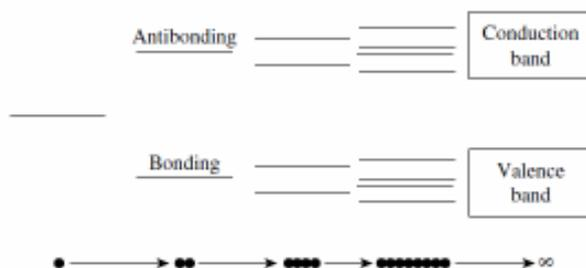
Figure 5: Illustration (extracted from <sup>31</sup>) of the energy levels from one atom to the bulk behavior and the forming of valence and conduction bands.
