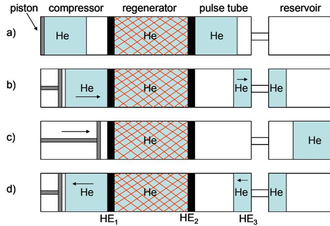
Figure 6: Schematic drawing of the PT cooler cycle containing the compressor, regenerator and pulse tube rooms. The He inside the pulse tube exchange heat with  $X_2$  (a). The piston moves periodically and pushes the He inside the compressor to exchange heat in  $X_1$  and He gas inside the pulse tube exchange heat in  $X_3$  (b). The He inside the pulse tube and the regenerator are never cross (c and d).
