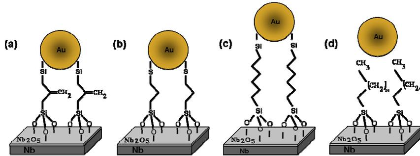
Figure 4: Au NP's attached by self assembled monolayer on top Nb superconductor film. (a) 3-methylpropane bis-trichlorosilane (diSilane), (b) mercapto propyl silane (MPS), (c) 1,6-Bis(trichlorosilyl)hexane (Hex diSilane) and (d) octadecyl trichlorosilane (OTS).
