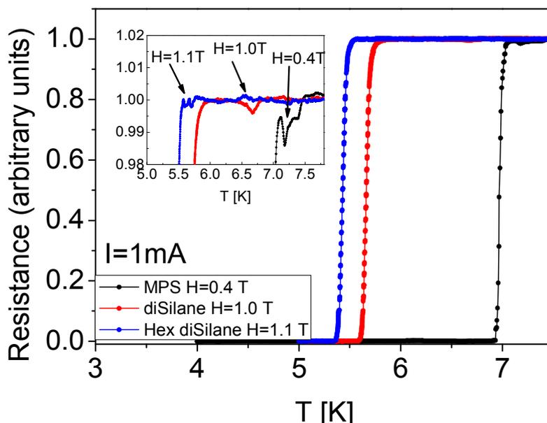
Figure 16: Normalized resistances of the Nb films as function of temperature for the three molecules used. The higher the magnetic field at which the peak effect is first observed the weaker the coupling of the molecule.
