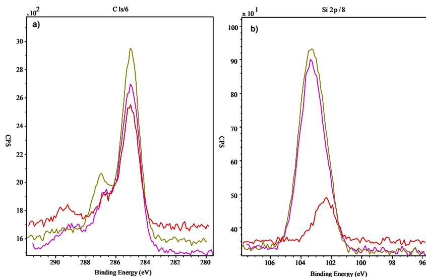
Figure 12: XPS measurement of Nb film clean (red), with monolayer (yellow) and after 10 Au NP's (pink) for Carbon at 285 eV correlate to C-C bond (a) and Silicon at 103.4 eV correlate with Si-O bond (b).
