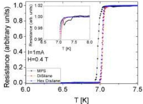
FIG. 3. (Color online) Normalized resistance of the Nb films as function of temperature. The molecules adsorbed on top of the film are DiSilane, Hex DiSilane and MPS. All measurements were performed at 0.4 T external, dc magnetic field. The inset shows a blow up of the peak effect area just below the Nb critical temperature. Only in the MPS system with the shorter length molecules a peak effect can be recognized.
