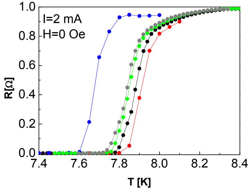
Figure 18:  $R(T)$  characteristics for 150nm Nb film: Blue- bare Nb substrate, Red- after diSilane adsorption and 10-nm Au NPs deposition.  $R(T)$  curves were then measured for the same sample, after partial removal of the organic layer and the Au NPs by plasma: Black- after 10 minutes plasma cleaning, Green- after 20 minutes plasma cleaning and Gray- after 60 minutes plasma cleaning. No effect of the plasma cleaning was seen on the bare Nb film.
