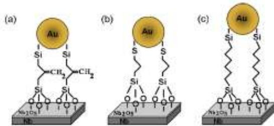
FIG. 1. (Color online) Schematic drawing of the experimental system. Cr/Au four-probe configuration contacts were evaporated on the Nb film. Self-assembled monolayers of three types of organic molecules were adsorbed on top of the sample. (a) 3-methylpropane bis-trichlorosilane, which forms a 3-nm-thick layer, (b) MPS, which forms a 0.5-nm-thick monolayer, and (c) 1,6-Bis(trichlorosilyl)hexane, which forms 4.5-nm-thick layer.
