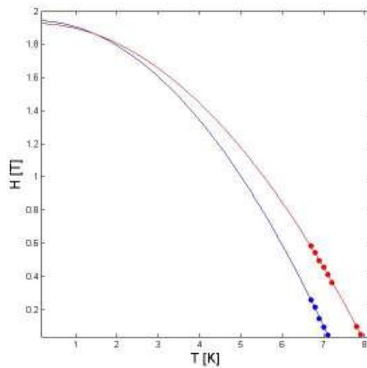
Figure 22: critical temperature as a function of external DC magnetic field perpendicular to the sample's surface for bare Nb film (Blue) and Nb adsorbed with diSilane molecule (red). The intersection of the fit curves may indicate of matching field.
