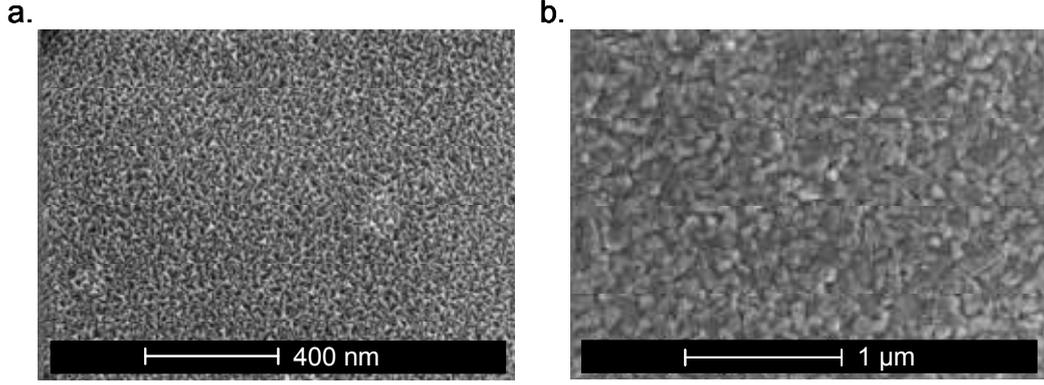
Figure 9: SEM pictures of Nb surface fabricated by e-beam evaporation (a.) and by sputtered (b.) techniques.
